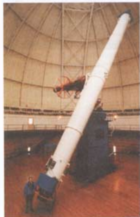
3-7 The world's largest refractor, with a 40 in. objective, is located at Yerkes Observatory in Williams Bay, Wisconsin. Because of the weight of the objective lens, a refracting telescope larger than this would not be practical.
