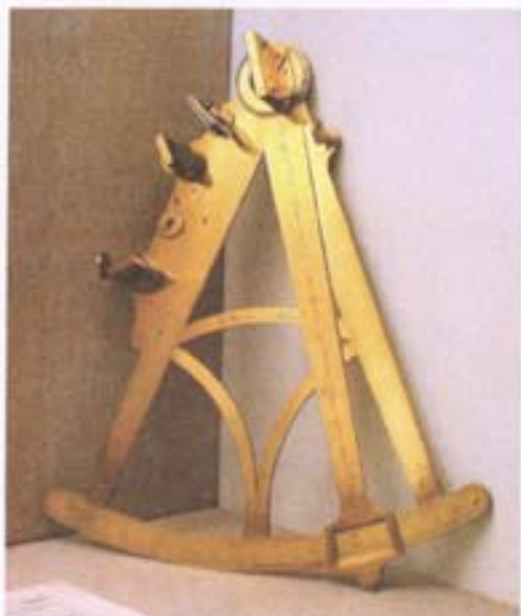
3-3 Octants were used to read the angle a star made with the horizon.
